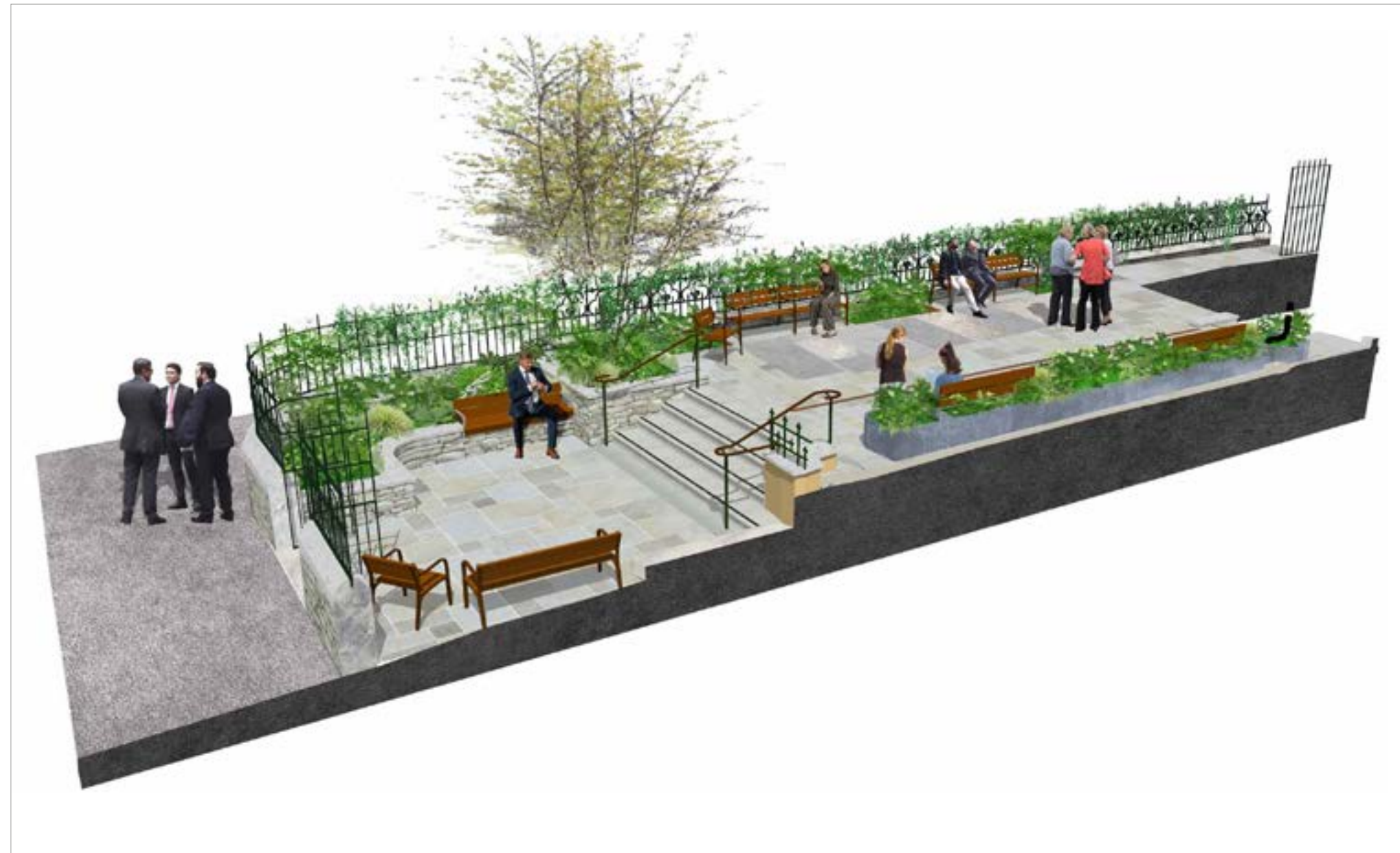
St Andrew Undershaft Churchyard: Integrating future-proof design with historic architecture, St Andrews Undershaft churchyard captures rainwater from the church's roof to store it in new planting beds. The scheme features permeable paving, more greenery, increased seating and offers a revitalised space for public enjoyment and biodiversity.
