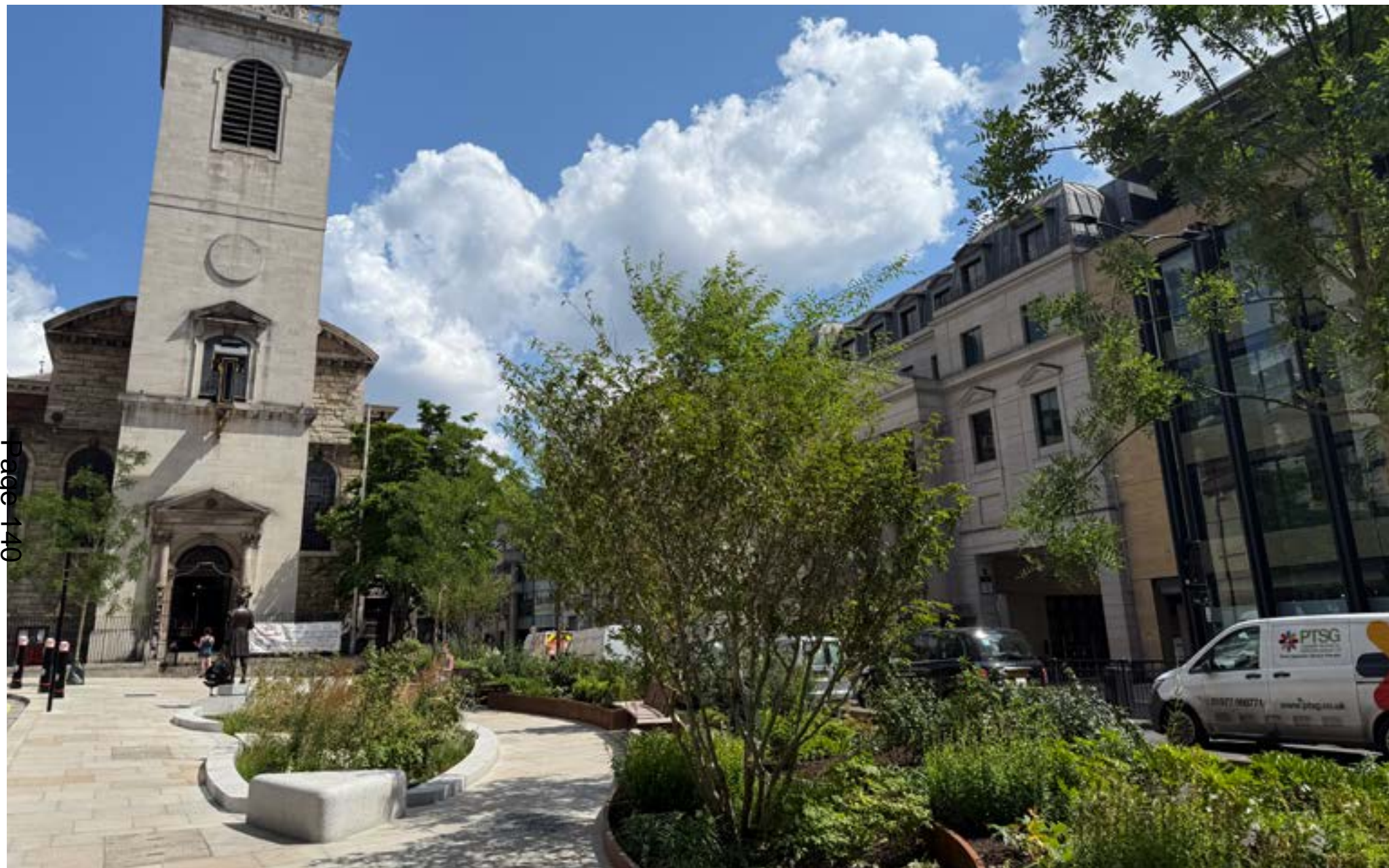
Little Trinity Lane: Flood resilience at Little Trinity Lane, which captures surface water running down Garlick Hill storing it in the beds to irrigate plants.
